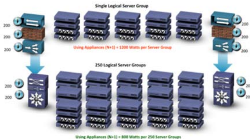
Figure 2. Data Center Virtual Services Reduce Load from 1200 to 800 Watts
